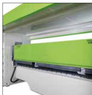
Folding beam in upper position before clamping.
