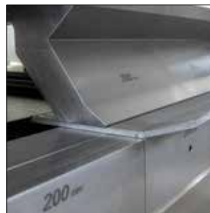
Power enough to fold up to 6 mm (0.236") mild steel.
