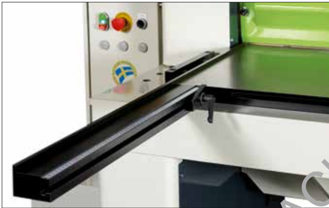
Squaring arm with or without T-groove and tilting stop. Available from 440 mm (17.3") to 3000 mm (118") for EVO , and 1000 mm (39.3") or 2500 mm (98.4") for RAPIDO .
