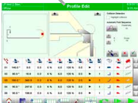
This function automatically calculates the folding sequence, detects collisions and visualises this to the operator.
