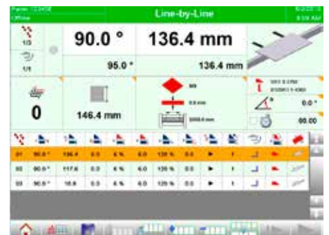
A third programming alternative is Line By Line. Set angles and dimensions and the machine will be ready to fold.
