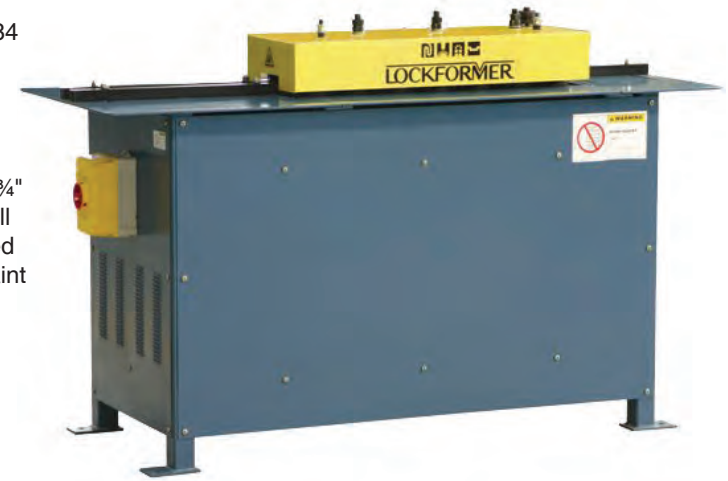
The auto-guide power flanger will create this right-angled flange See pg. 12
